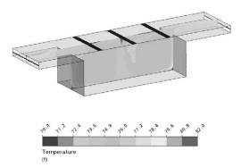
Figure 7: Contour plot showing the average temperature in a bar-section for a still day and an external air temperature 2°F below the internal set point.
