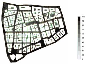
Figure 2: Percentage of exceedence for a wind speed greater than 0.5m/s (100fpm)
