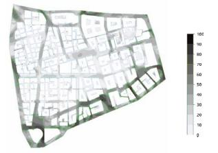
Figure 3: Percentage of exceedence for a wind speed greater than 2m/s (400fpm)
